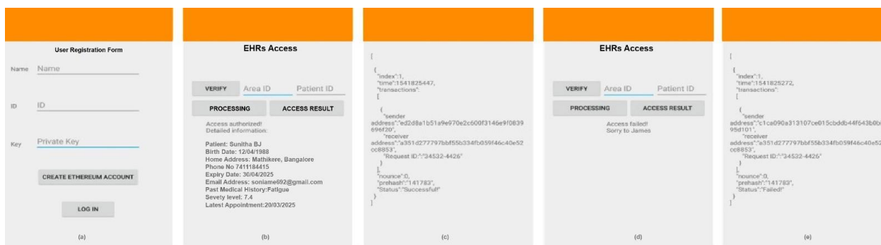
Figure 12. Visualizing EHR access outcomes on Android devices: 12.a) Registering a user with an Ethereum account, 12.b) EHRs access results of an authorized user, 12.c) Log of approved EHR access transactions, 12.d) EHR results obtained by an unauthorized user, and e) Record of unauthorized access to EHRs.
